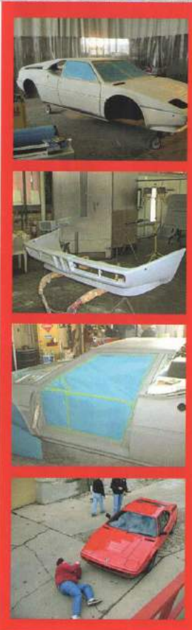
ProjectM1 was media blasted and then sent to the bodyshop for plenty of body prep (see article!) before painting - eventually! New ‘European’ bumpers were sourced to replace the ugly federalized US ones. Menno also paid a visit in his red M1 to allow bodyshop owner Bob Bennett to take photos to ensure the paint/trim finish is 100% accurate
