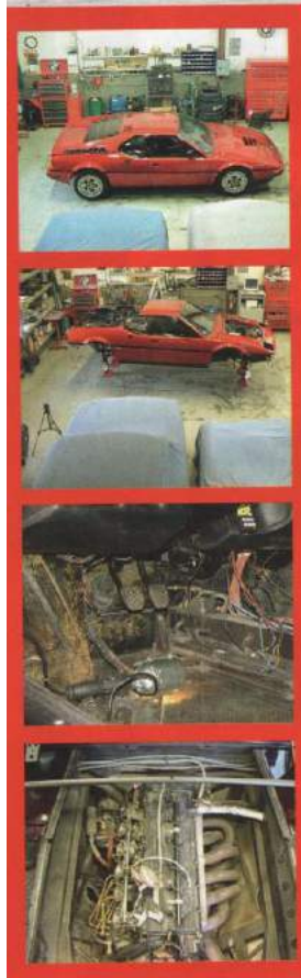
Menno's donor M1 was delivered to the WerkShop complete with its 'dadgy' Candy Apple red paintwork and aftermarket alloy wheels. The car was then completely stripped. Here we can see the driver's side footwell area with all carpets and soundproofing removed and the M88 engine before it is removed from the shell
