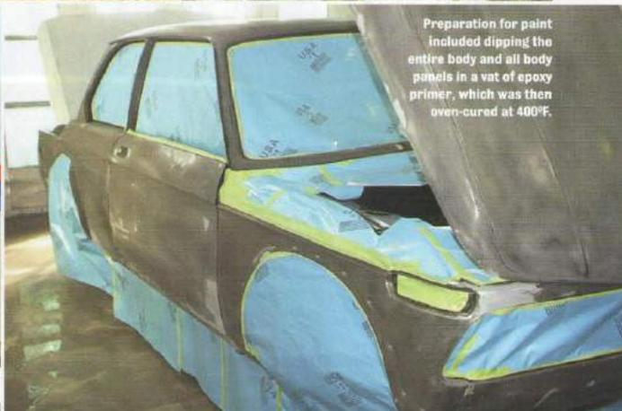
Preparation for paint included dipping the entire body and all body panels in a vat of epoxy primer, which was then oven-cured at 400°F.
