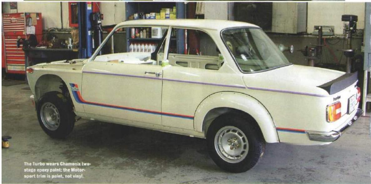
The Turbo wears Chamonix two-stage epoxy paint; the Motorsport trim is paint, not vinyl.
