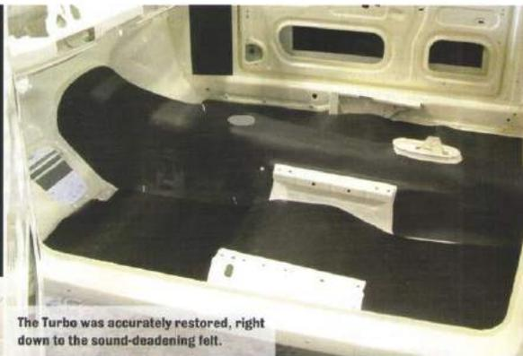
The Turbo was accurately restored, right down to the sound-deadening felt.
